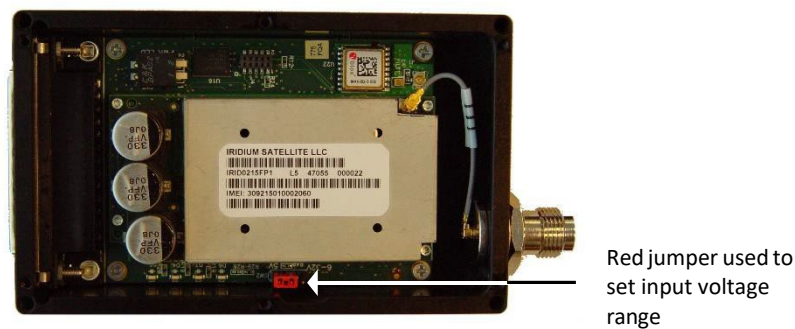
Figure 2: Power Input Setting for the A3LA-R
