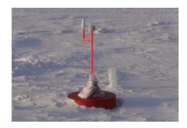
The hull is constructed of aluminum with an lonomer foam collar for floatation. The tubular hull is intended to be placed into a hole drilled in the ice, which provides excellent stability. The design is compact and light to allow for simple deployment.
