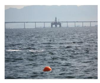
Scientifically, iSPHERE behaves like a maximum leeward drift object in the water. The force of the wind against the exposed surface of the buoy causes it to move through the water in a generally downwind direction. The resultant motion of the buoy is made up of the leeway drift and the movement of the upper layer of the ocean caused by the surface currents. iSPHERE has been shown to drift in the direction of the oil slick closest to the ocean's surface.
