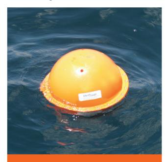
iSPHERE is a low cost expendable Lagrangian drifter with a state-of-the-art data acquisition system which collects real-time sea surface temperature data with an accurate thermistor as well as GPS positional data.
