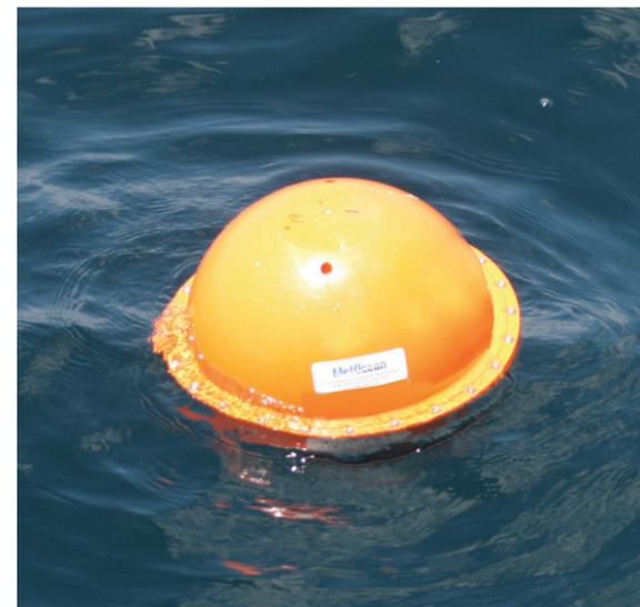
**iSPHERE is a low cost expendable Lagrangian drifter with a state-of-the-art data acquisition system which collects real-time sea surface temperature data with an accurate thermistor as well as GPS positional data.**
