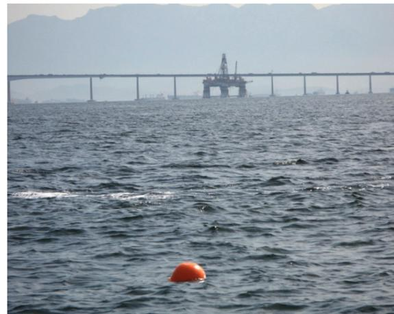
Scientifically, iSPHERE behaves like a maximum leeward drift object in the water. The force of the wind against the exposed surface of the buoy causes it to move through the water in a generally downwind direction. The resultant motion of the buoy is made up of the leeway drift and the movement of the upper layer of the ocean caused by the surface currents. iSPHERE has been shown to drift in the direction of the oil slick closest to the ocean's surface.
